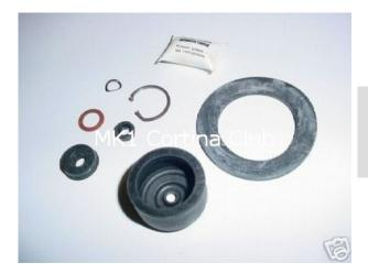
Master cylinder kit (SP1963)will also be used as brake kit suitMaster cyl kit drum brake & 5/8 disc brake m/cyl
